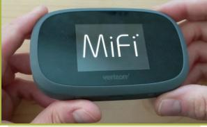
"MiFi" is a wireless router that acts as a mobile Wi-Fi hotspot allowing your devices to connect to the internet.
